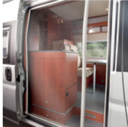
The new fly screen sliding door is continuously adjustable.
