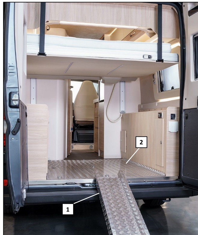
Access ramp and metal tray for the V 635 HB (sample illustration)
