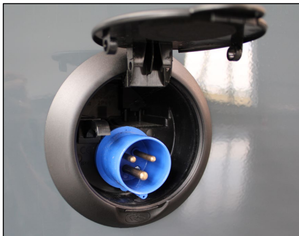
230-V CEE power supply connector on the outside of the vehicle (sample illustration)
