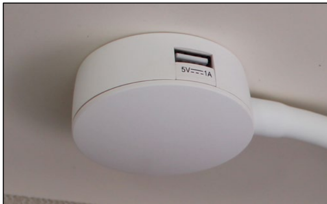
USB port in the base of the LED reading light
