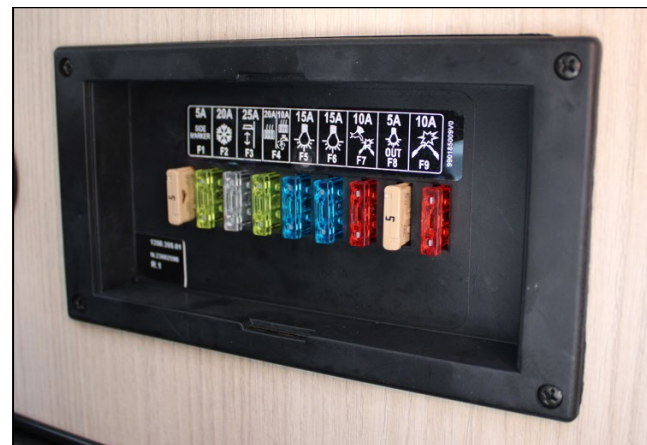
12-V fuse box switch under the driver seat (sample illustration)
