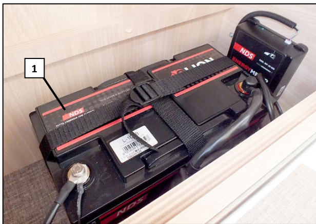
Optional lithium battery with meter with display (sample illustration)
