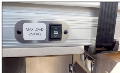
Control switch for drop-down bed, rear
