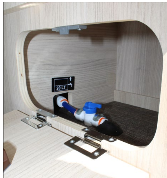
Drain valve for fresh water reduction to 20 l in the V 635 EB/HB (sample illustration)
