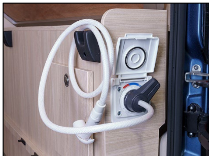
Additional shower connection in the V 635 EB
