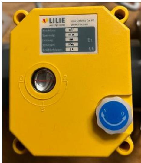
Electric on the waste water tank drain valve (sample illustration)
