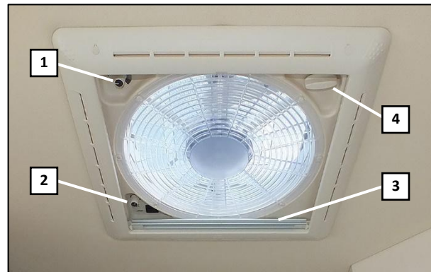
Roof vent with blackout blind
