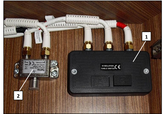
“A/B” channel switcher and signal distributor (example)
