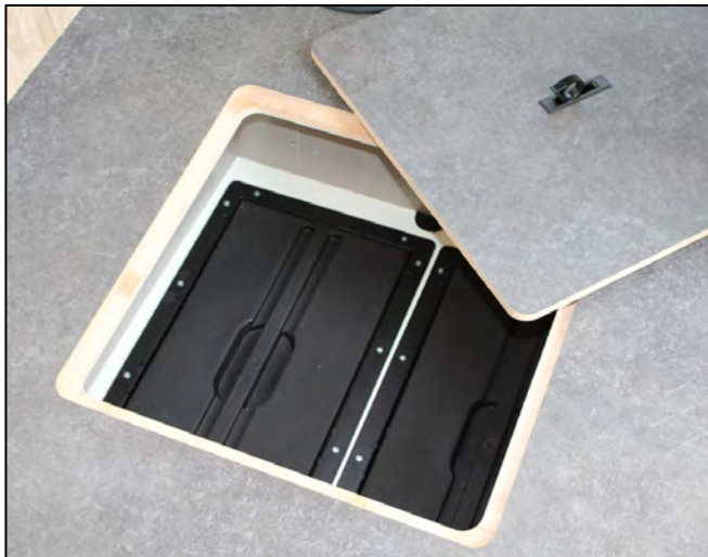
Superstructure battery in the double floor (sample illustration)
