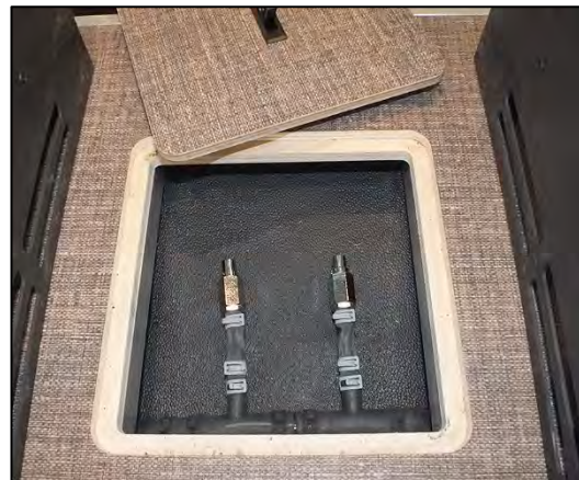
Connectors for the ALDE heated floor mat (sample illustration)
