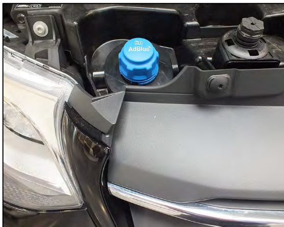
AdBlue filler opening in the front section of the engine compartment (sample illustration)
