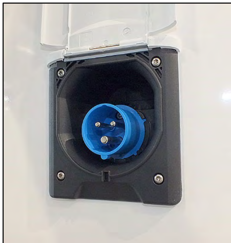
CEE power supply connector (230 V) on the outside of the vehicle (sample illustration)
