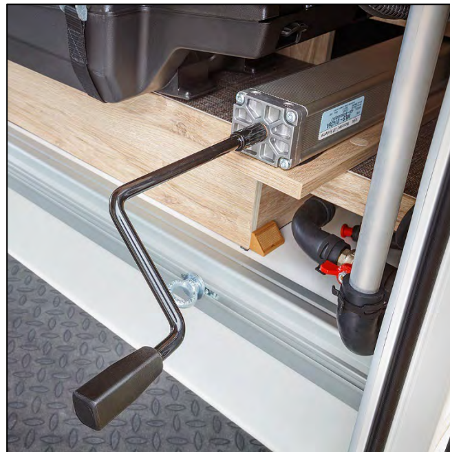
Manual height adjustment mechanism for the central bed (sample illustration)
