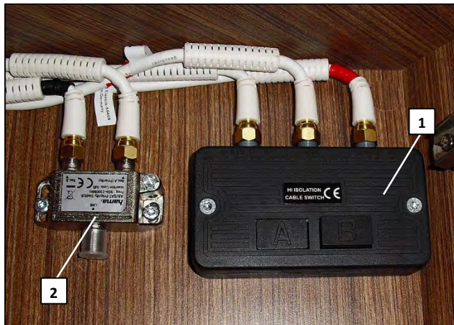
“A/B” channel switcher and signal distributor (example)
