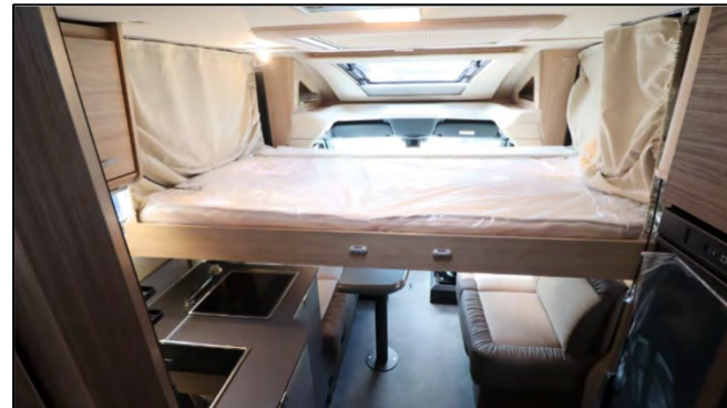
Manual drop-down bed in sleeping position (sample illustration)
