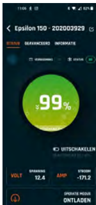
Display of the state of charge of the lithium battery on the smartphone (sample illustration)
