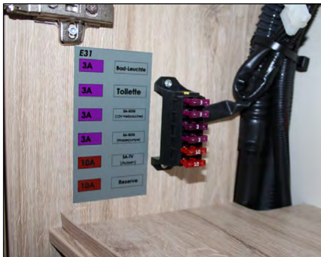
Additional fuse holder underneath the wash basin (sample illustration)
