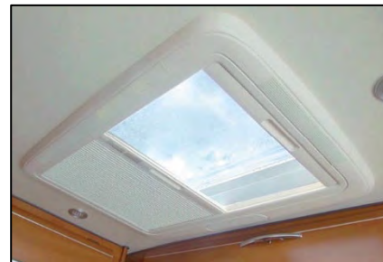
Blackout blind on the roof light (sample illustration)
