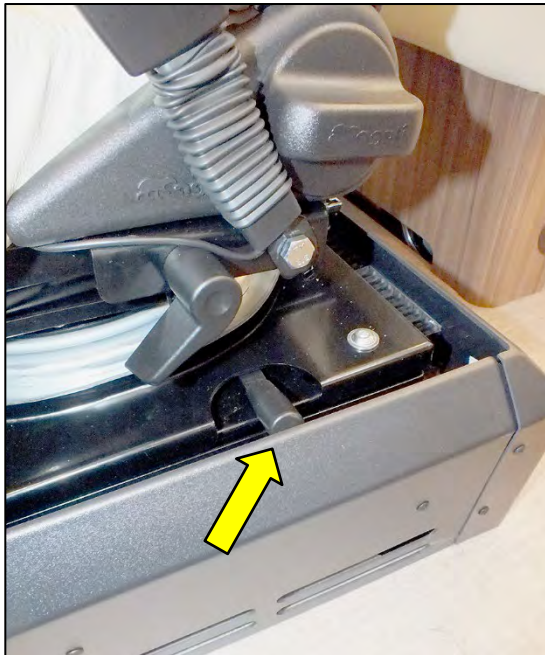
Locking lever on the base of the driver seat (sample illustration)
