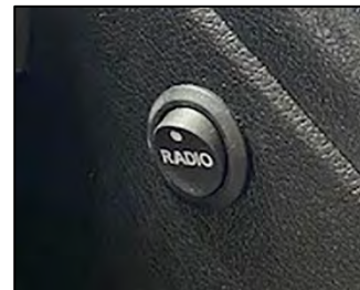
ON/OFF switch for the multimedia system (sample illustration)
