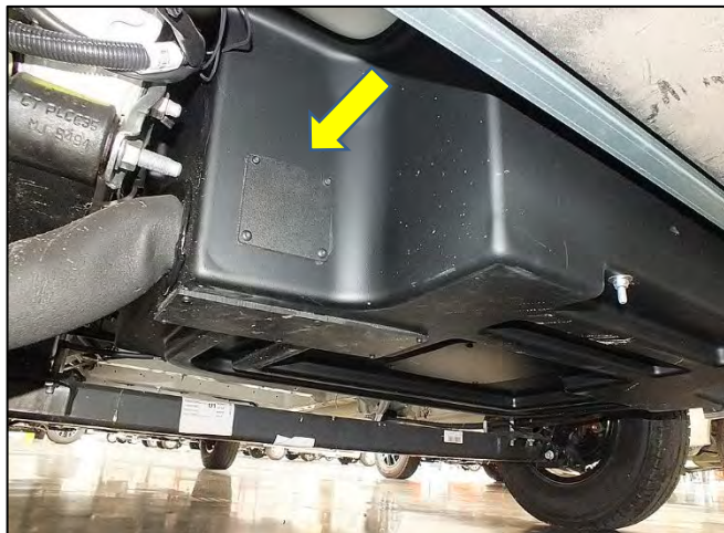
Service panel on the outside of the waste water tank (sample illustration)
