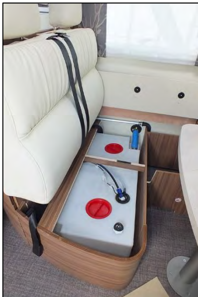
Fresh water tank in the seat compartment of the crosswise bench (sample illustration)
