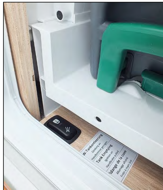
Push button for draining the waste water tank of the PT/PRS 675 SB (sample illustration)
