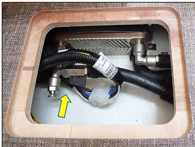
ALDE heat exchanger (sample illustration)
