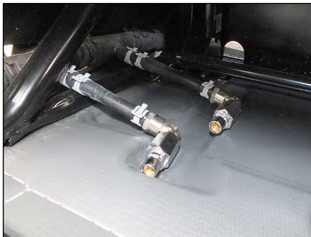
Connectors for the ALDE heated floor mat (sample illustration)
