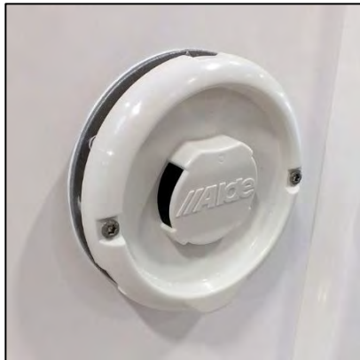
Ventilation opening for the heating, on the outside of the vehicle (sample illustration)
