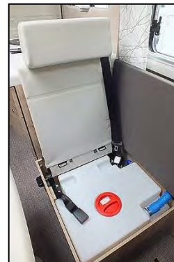
Fresh water tank in the lengthwise bench (sample illustration)
