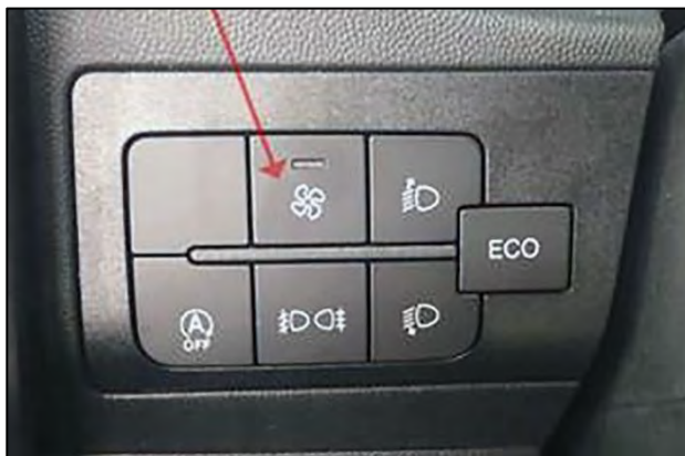
“Fan” button for activating the heat exchanger (sample illustration)
