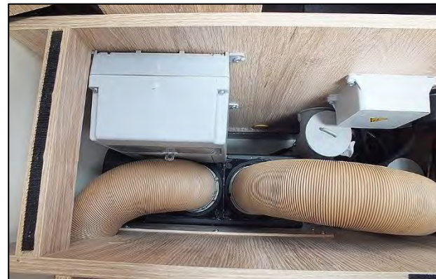
TRUMA heat exchanger in the seat box of the lengthwise seat (sample illustration)
