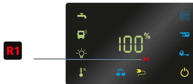
Warning signal for the waste water tank
