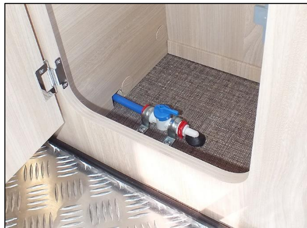
Drain valve for fresh water reduction to 20 l in the V 635 EB/HB (sample illustration)
