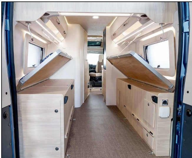
Slatted bases folded up and secured, additional storage units and intermediate floor removed (sample illustration)
