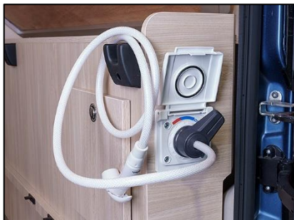
Additional shower connection in the V 635 EB
