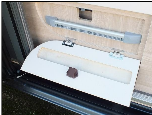
Attachment rail on the outside of the kitchen unit
