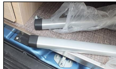
Additional crosswise support tubes in the V 635 HB
