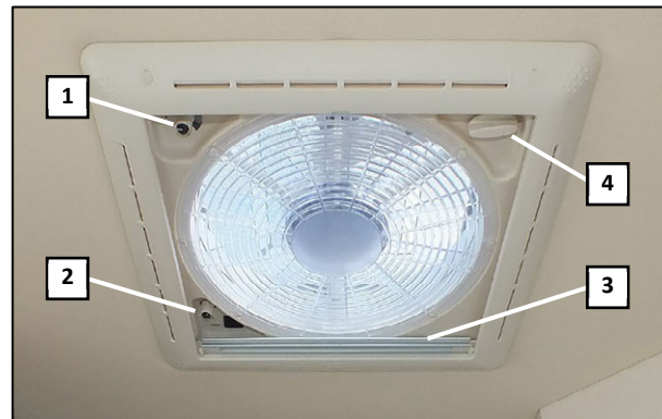
Roof vent with blackout blind
