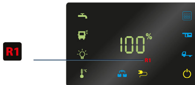
Warning signal for the waste water tank
