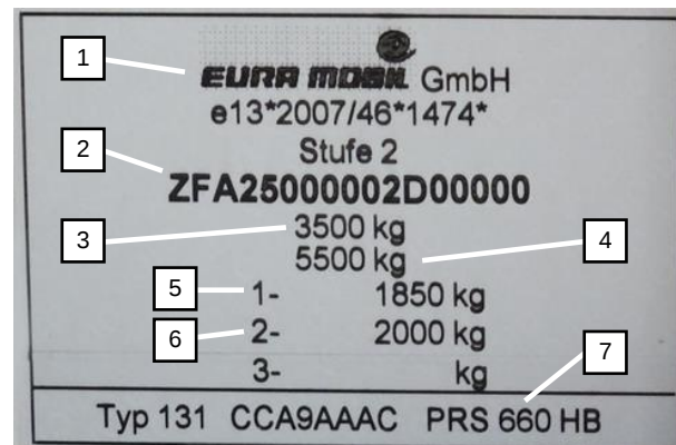
Superstructure type plate (example)
