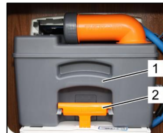
Waste holding tank
