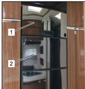
Oven above the refrigerator
