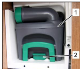
Waste holding tank (sample illustration)
