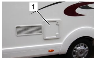
Cover holding tank
