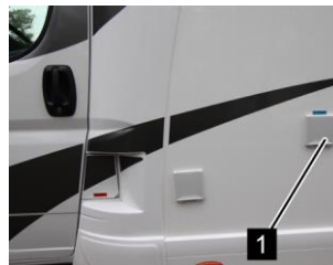
Filling connection fresh water tank
