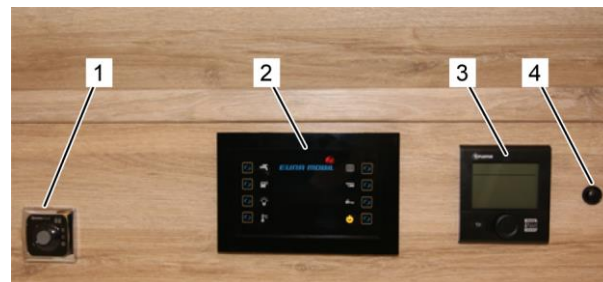
Operating elements above the superstructure door
