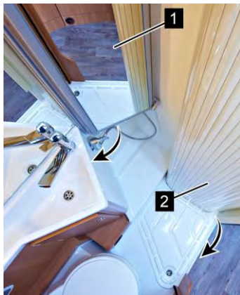
Conversion to shower cubicle
