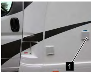
Filling connection fresh water tank
