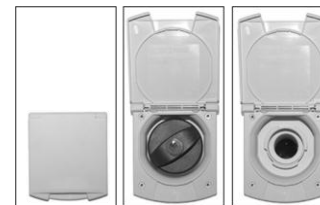
Topping up with fresh water
