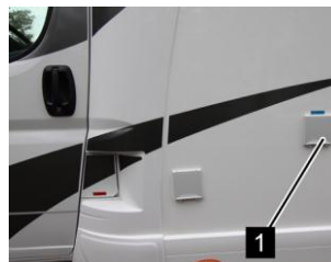
Filling connection fresh water tank
