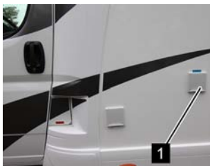
Filling connection fresh water tank
