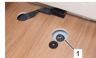
Drain cock fresh water tank
