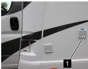
Filling connection fresh water tank
