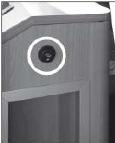
Operating control for electric boarding step
