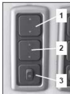
Height-adjustable seat and light switches
