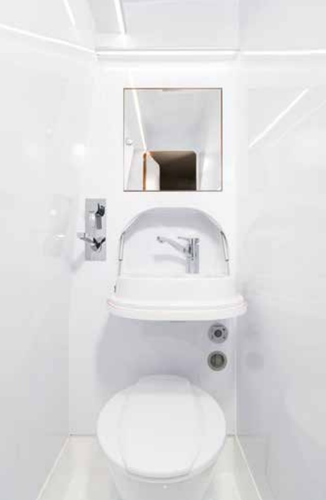
Inside the spacious lavatory is a folding sink, and behind the mirror is a cabinet with a 230 V outlet. The toilet bowl is ceramic.
