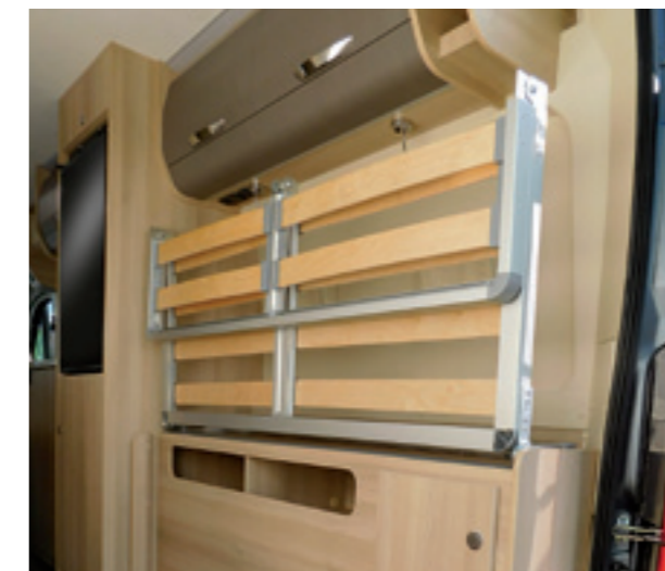
2 Prestige model: the bed base folds to leave the wall units accessible.
