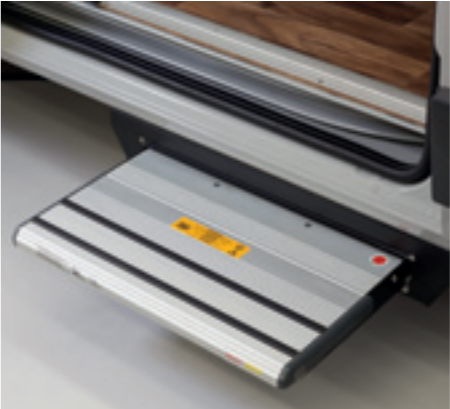
Electric living quarters access step.
