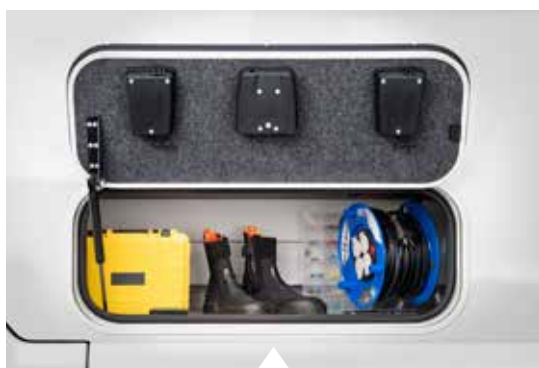
Outside hatches without any thermal bridges Everything is accesible in the dobule floor.
