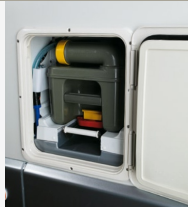
Wc combinato Thetford e nautico (1002) Thetford Cassette toilet (1002) Wc combiné Thetford et nautique (1002) WC mit Thetford Kasette (1002) Wc " combinado " Thetford y náutico (1002)
