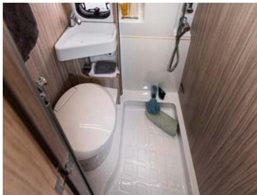
Lowered shower tray: the water does not flow into the toilet area.
