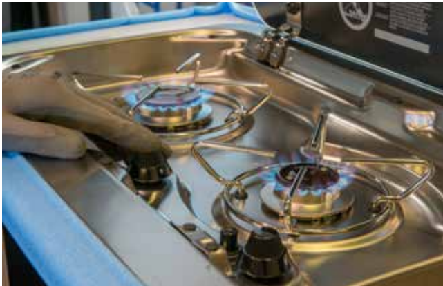
Test on operation of the gas pipes.
