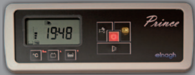
Central control console with LCD screen. Interior and exterior temperature sensors.
